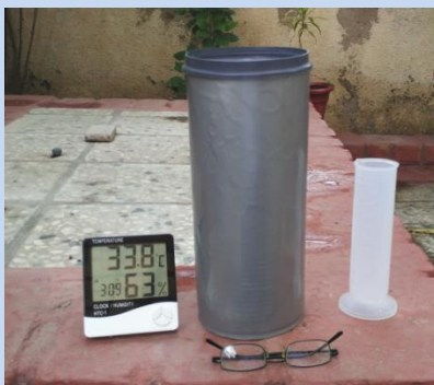
Temp./Humidity Measuring Unit , Raingauge & Measuring Cylinder
